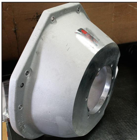
>> We want to go nines, so a SFI certified bell housing is required, Dynamic uses JW for all of its bell housings and transmission cases.
