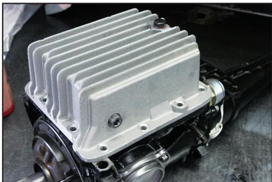
>> A deep trans oil pan is standard on the Mighty Mite M2 and Dynamic recommends filling it with the company’s proprietary synthetic transmission fluid. It worked with a major oil manufacturer to develop a blend of fluid that withstands severe temperatures and Dynamic recommends its use in the C4.
