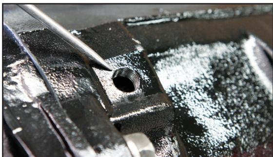
>> Apuzzo added a thread hole to the vent on our Mighty Mite M2 so we can run a catch can to prevent spillage during wheelies.
