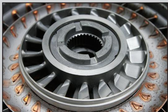
Opening up the torque converter reveals quite a few parts and pieces. Pictured is a stator that the TCT experts selected specifically for this application. The pump and turbine are furnace braised for durability and TCT includes a billet steel hub and a billet steel pump impeller in the Renegade torque converter line. All TCT torque converters come standard with rollerized bearings no matter what level of performance.
