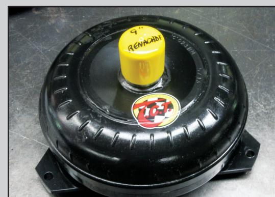
We opted for the 9-inch Renegade torque converter that has a billet front cover. It is rated to over 1,500 hp, which is far more than our little supercharged combination will be putting out.
