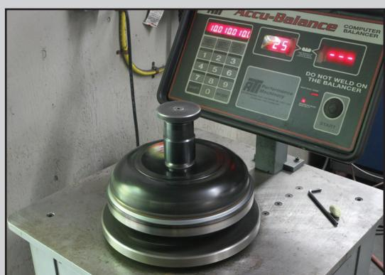
The torque converters are modified, built, and welded in-house. TCT also balances each torque converter and pressure checks them to ensure the highest quality and best performance.
