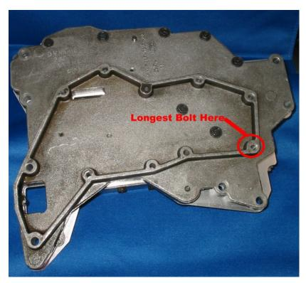
8. With all the bolts installed, tighten them to the following torque specs:
