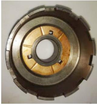
13. Place the Rear Drum over the drive hub assembly, interlocking the tangs of the 8 Pinion Planetary with the slots in the drum. Make sure the tangs fully seat in the drum slots.
