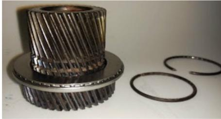
7. Install one of the Sun Gear snap rings over the small end and down so that it seats on the groove just above the roller bearing.
