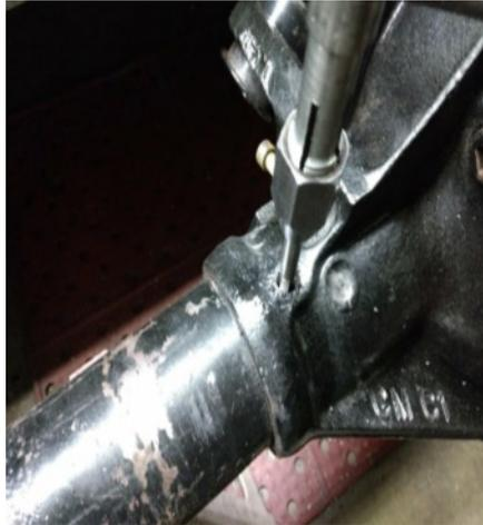
6. Once tapping has been completed, thoroughly clean the housing and tubes of metal chips.
