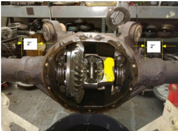
3. Determine the locations for your pins by spacing them equally around the cleaned casting. Some housings will use three per side, others can use the full four. Mark the locations for drilling using a Sharpie or paint pen.
