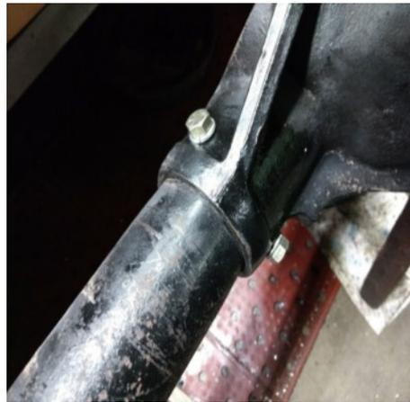
Once all bolts have been installed and torqued you can proceed with the rest of the axle housing assembly.
