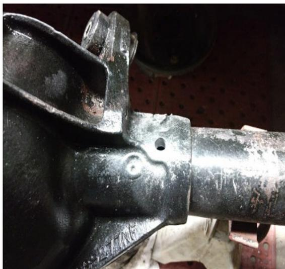
Drill completely through the housing and the axle tube assembly.
