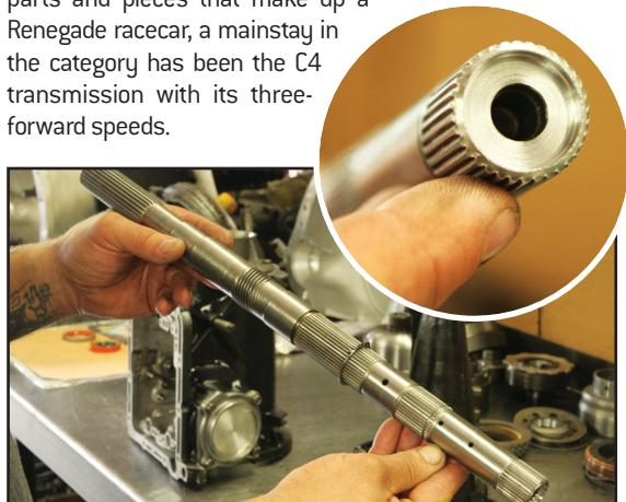
>> The OEM output shaft gets checked on the lathe for straightness and once the team determines it is an acceptable shaft, it is machined for clearances. All of the bushing areas are polished and the end (inset image)—where the output shaft meets the input shaft—is machined down to eliminate the shafts from beating each other up.
