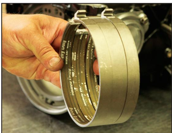
>> The first component to be installed in the C4 case is the reverse band. Dynamic uses a Kevlar one for durability.
