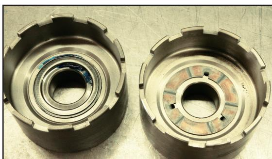
>> Dynamic replaces all thrust washers (right) with Torrington roller bearings (left). This helps efficiency and durability in high-performance applications. It requires a significant amount of work on a lathe to trim and modify the internals to accept the Torrington bearings.
