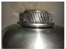
9. With the Sun Shell/Sun Gear Assembly facing upward, Place the 8 Pinion Planetary onto the large gear of the 2.20 Sun Gear.
