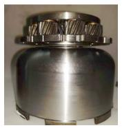
10. Install the small Roller Bearing into the recess of the 8 Pinion Planetary
