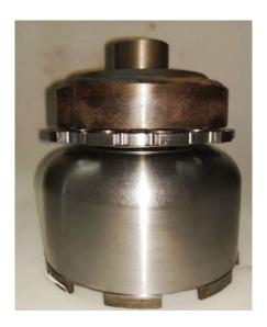
12. Now install the stock 3 tang thrust washer into the rear drum. A little Transgel or Vaseline under the washer will hold it in place. A Machined & Rollerized drum is available at extra cost
