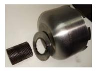
5. Thoroughly clean the Sun Shell and the thin washer. At this time you may replace your Sun Shell with one of Dynamic's Polished Lightened Sun Shell's P/N DA4DS1
