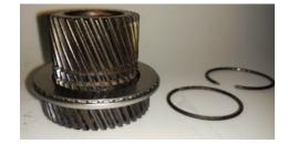
7. Install one of the Sun Gear snap rings over the small end and down so that it seats on the groove just above the roller bearing.
