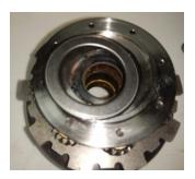
11. Now Place the new Welded Planetary Hub over the 8 Pinion Planetary, rotating to mesh the gears.
