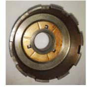
13. Place the Rear Drum over the drive hub assembly, interlocking the tangs of the 8 Pinion Planetary with the slots in the drum. Make sure the tangs fully seat in the drum slots.
