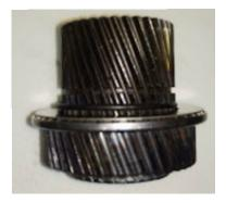
8. Now, place the stock Sun Gear Washer over the small end of the gear. Then install the sun Shell onto the Sun Gear. Lock it in place using the second snap ring inside the shell. Be sure it seats in the second groove firmly.
